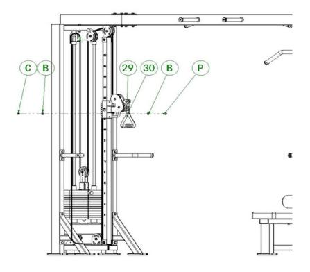
Schematic diagram of wire rope routing
