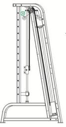
Left side frame wire rope alignment diagram
